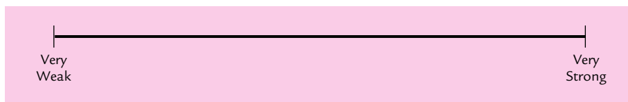
FIGURE 9-3 Rating scale formatted with no numbers. End points are labeled, and participants place marks on the line to indicate their responses.
